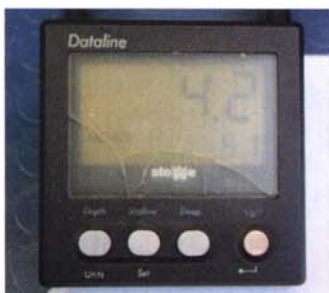
UV rays cracked this screen cover
